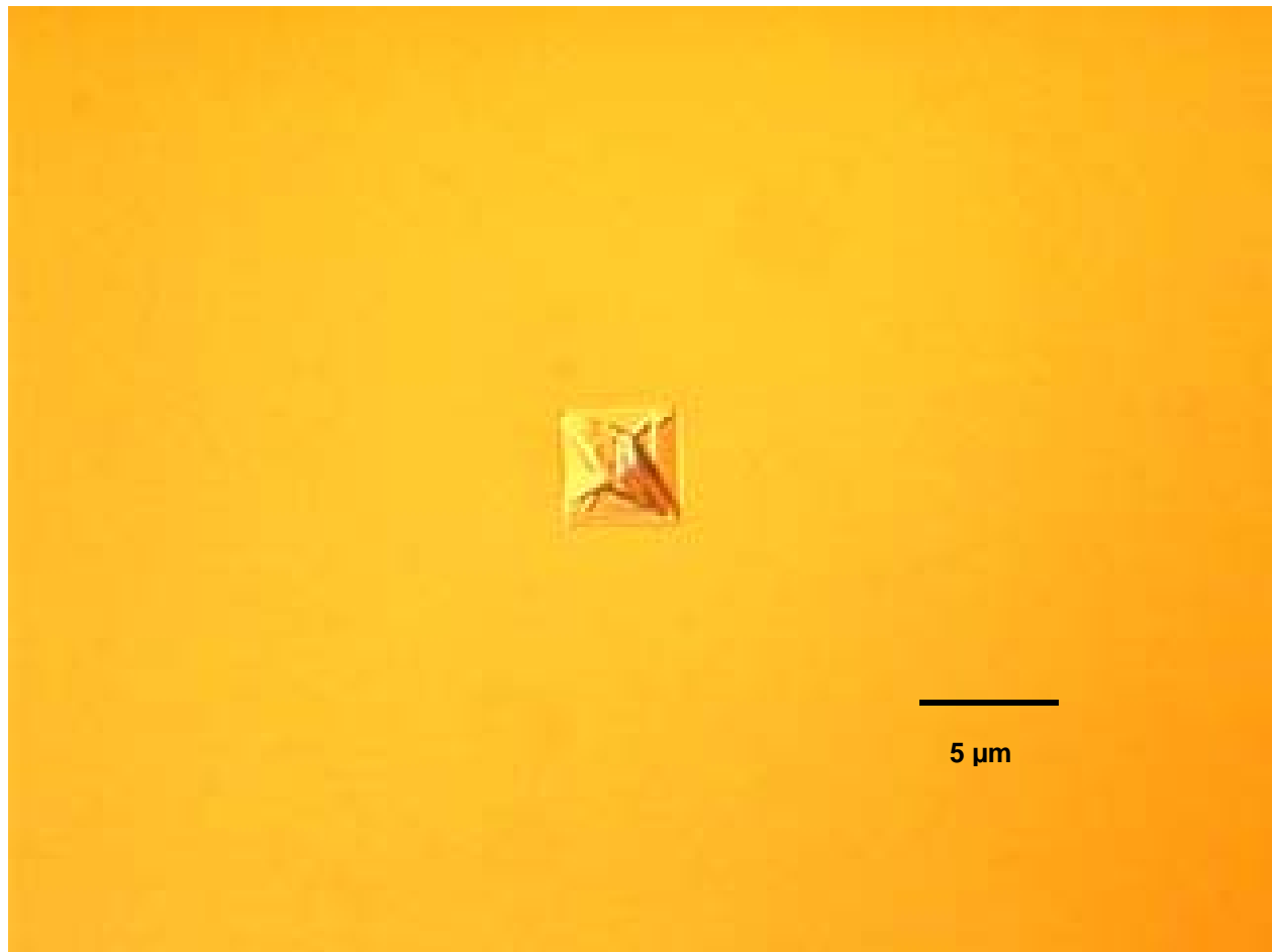
Figure 10 Composite Defect of polysilicon growth and stacking faults. Magnification 500 times by Nomarski Interference Microscopy. Approximate SSIS image event size \gg 1.0 \mu\text{m}
