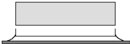
Figure 2 Mode 2 — Interface Failure: Die-to-Adhesives
